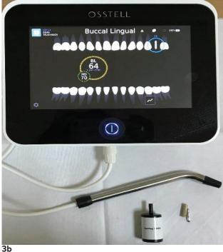
**Figure 3.** a) SmartPeg connected to the dental implant and measurement of primary stability of the dental implant; b) Osstell Idx device
