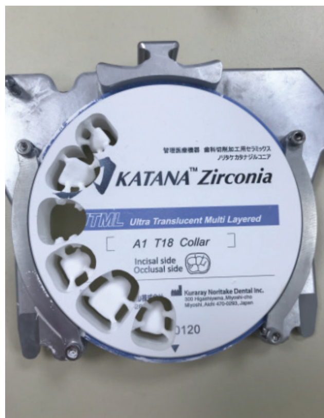
Figure 2. A zirconium 18 mm, ultra-translucent multi-layered disk KATANA (Kuraray Noritake Dental Inc., Japan)
