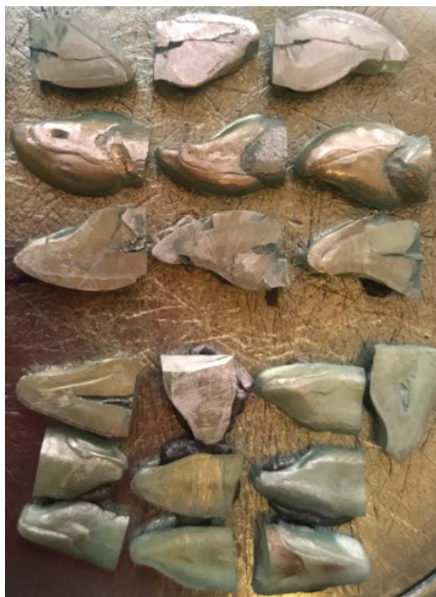
Figure 3. The specimens fixed onto an experimental tray and covered with gold particles through electro- vacuum metallization.
