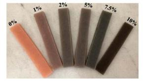
Prepared samples for flexural strength testing
