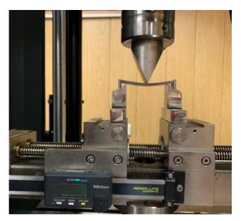
Figure 2. Zwick Roell for the flexural strength test.
