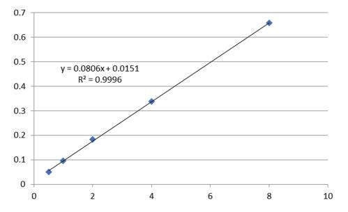
Figure 2. Calibration curve of mycophenolic acid (n=5). X axis: standard MPA concentration (0.5–8 µg/ml); Y axis: peak area ratio.
