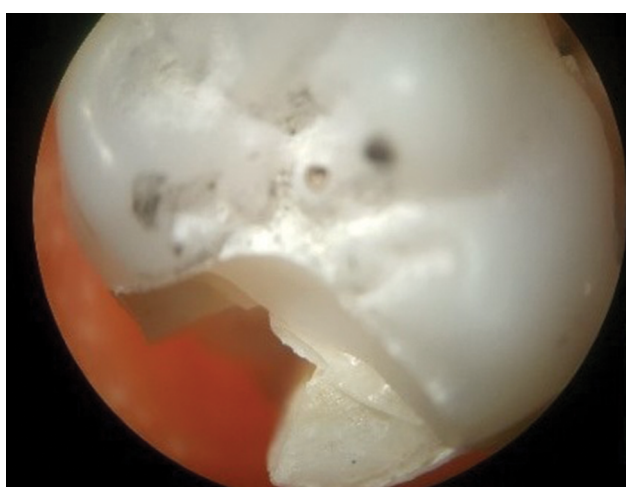
Figure 5. Stereomicroscopic image \times 10 presenting type (mixed type failure below the CEJ) failure mode of endocrown specimen.
