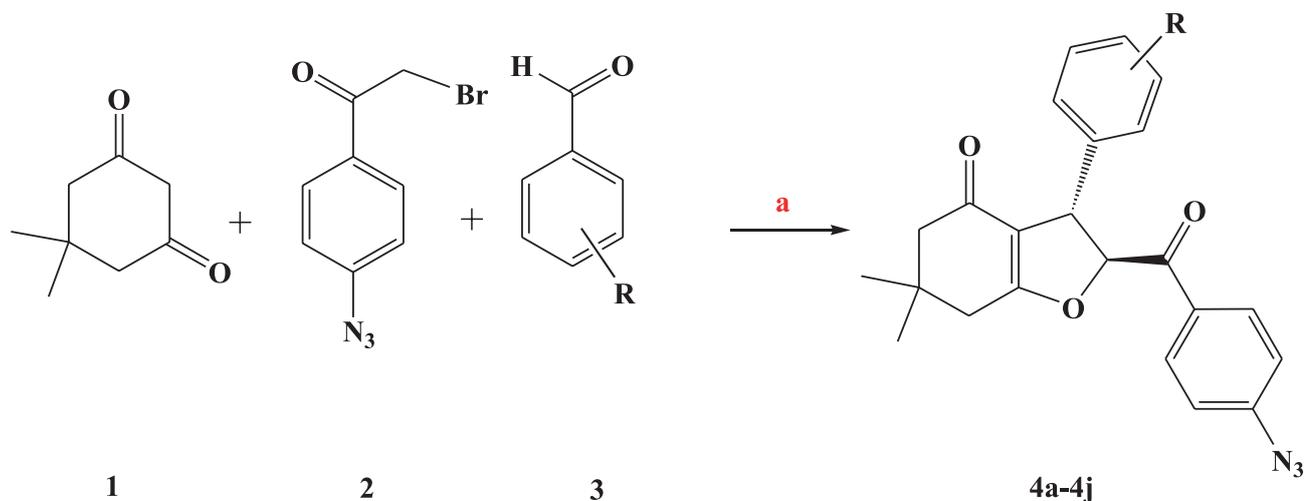
Reaction Scheme 1. Reaction and conditions: a) Acetonitrile, pyridine, 60-70°C 3.0 h; and A/3.0 h, TEA, 60-70°C, 3.0 h.
