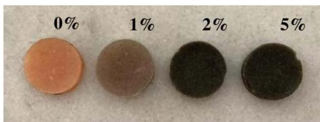
**Figure 3.** Preparation of acrylic discs containing selected C-phycoyanin (containing the highest percentage of clinically acceptable flexural strength).
